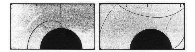
Fig. 1a & 1b: Shadow pictures of the unsteady fiow field around a cylinder with radius 5 cm at time 104  $\mu$ s (left) and at time 284  $\mu$ s (right) after the impact of the incident shock (M<sub>0</sub> = 1.38, p<sub>0</sub> = 0.985 bar) at the left stagnation point. In the right figure the diffraction phase is nearly terminated. The reflected shock and the Mach stem travel away from the cylinder and leave the test section.
