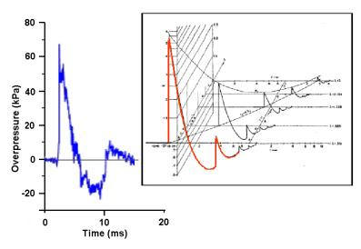
Comparison of blast waveforms as generated by a prototype Advanced Blast Simulator (blue) with the classical solution from Brode (red).
