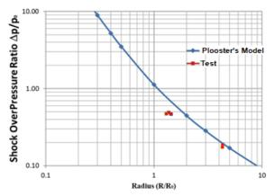
Figure 1: comparison between Plooster's model to test data
