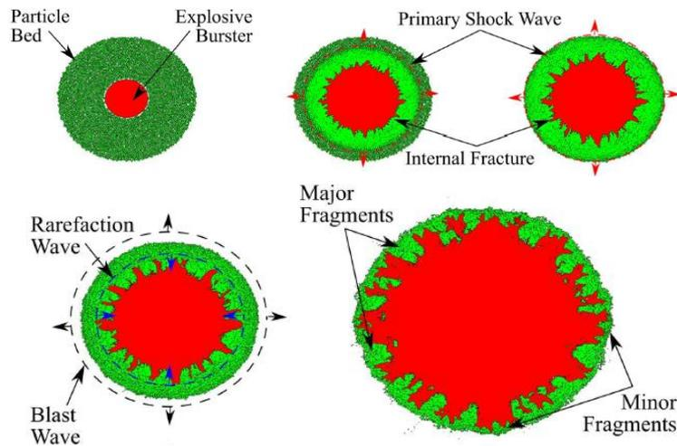
Figure 1: Mesoscale multiphase simulation results of the explosive dispersal of a layer of brittle ceramic particles producing a bimodal fragment size distribution.
