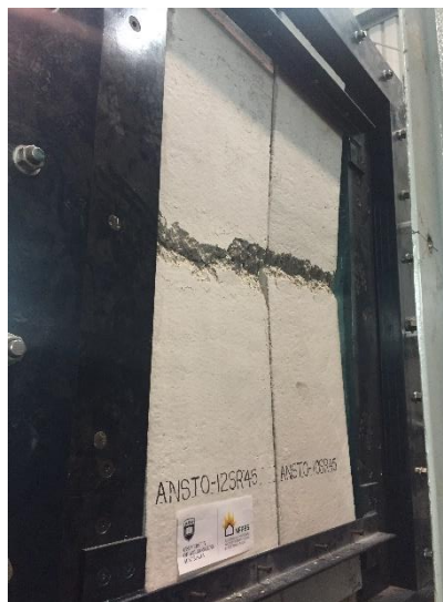
Figure 1. View of damaged RC panels after testing in the blast simulator.
