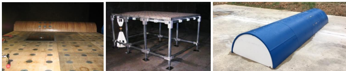
Figure 1: Non deformable hemi-cylindrical structures (IRSN, left – ISL, right) – IRSN BlastS table (centre)
