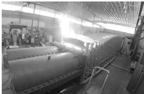
Figure 1: Blast at Driver End of ABS During ProtectiFlex™ Wall Panel Test
