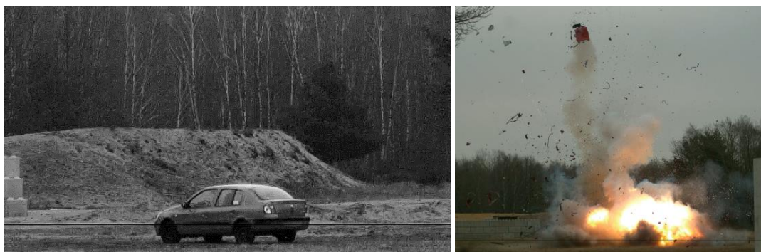
Figure 1: Flying fragments distribution after VBIED tests [Sielicki et al. (2021)].
